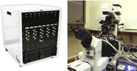
Figure 1 Compact L200 control cabinet, 27" H x 21" W x 26" D (left). L200 installed on a Nikon TE2000 inverted confocal microscope (right).
