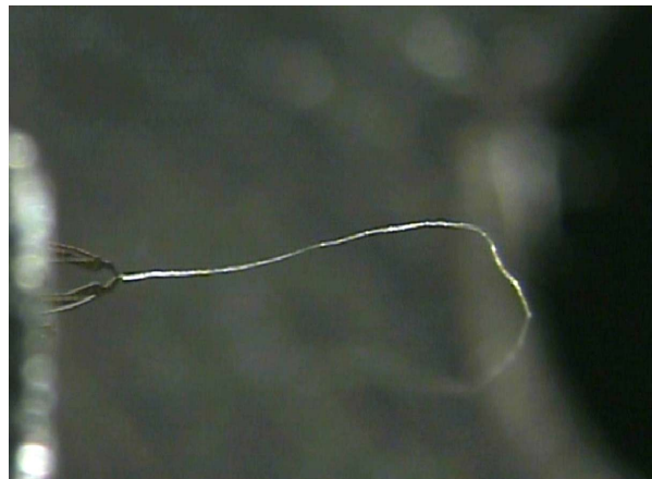
Figure 5 A MEMS gripper holding a free collagen fiber.
