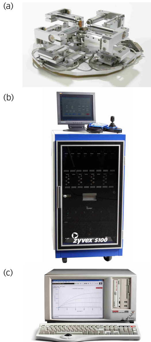
Figure 1 (a) KZ100 head unit with end-effectors installed. (b) Zyvex KZ100 Controller. (c) Keithley 4200 Semiconductor Characterization System.
