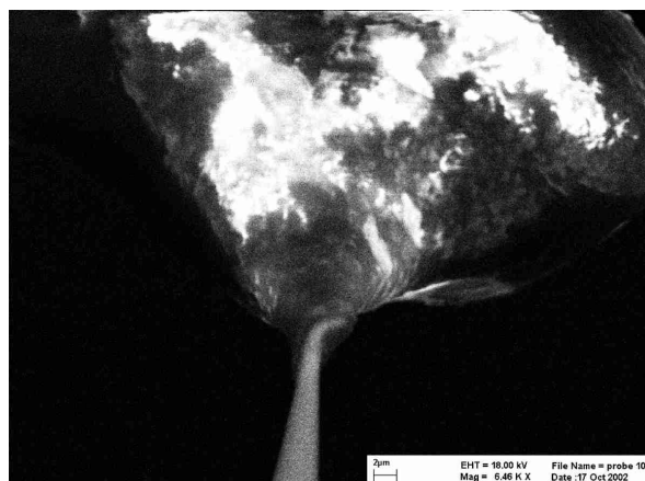
Figure 5 The tungsten wire submerged in the acrylic adhesive.
