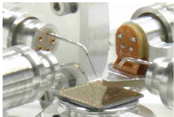
Figure 1 Zyvex S100 Nanomanipulator can function as a nano- and microprobe and is an ideal tool for dielectric breakdown voltage measurement.
