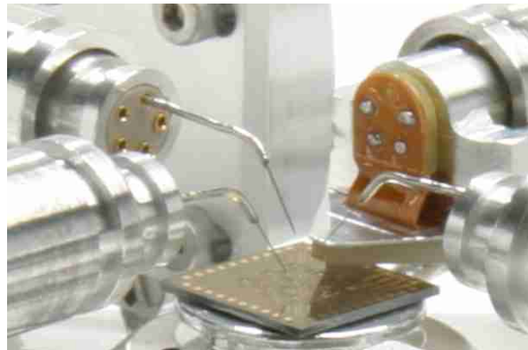
Figure 3 Microgripper end-effector interface
